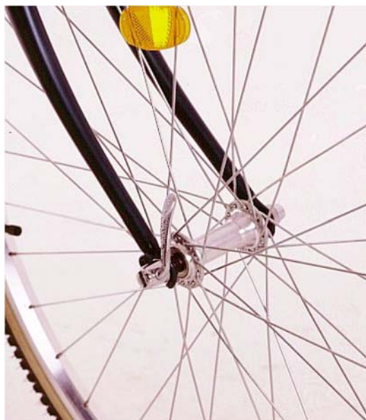
Figure 7 Quick Release Incorrect Position—Example 2
