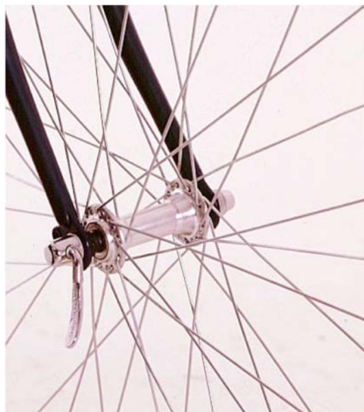
Figure 6 Quick Release Incorrect Position—Example 1
