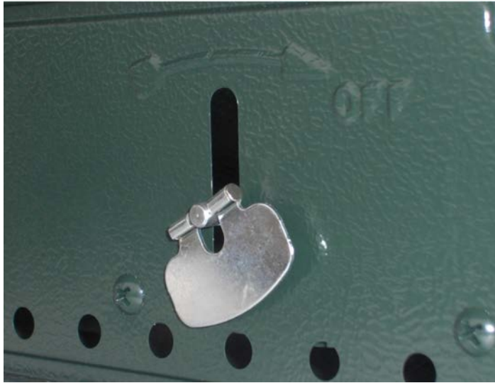
Figure 7 Auxiliary Burner Control
